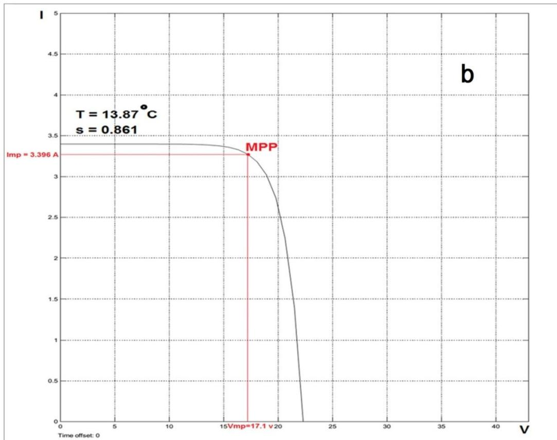
**Fig. 7.** Simulation: a) simulation of MSX-64 solar panel; b) I-V curves for maximum performance of the MSX-64 panel at the optimal location in Kermanshah Province
