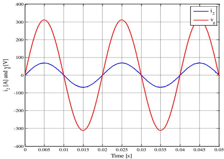
**Fig. 6.** Current and voltage of grid
